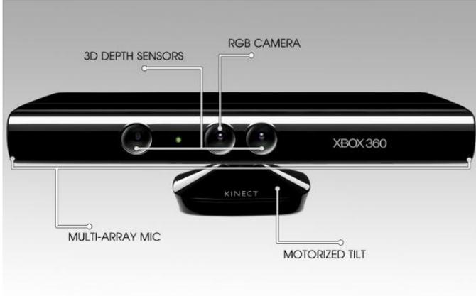
Fig. 2 The Kinect sensor
