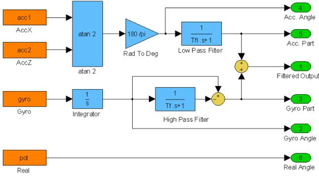
**Fig. 3 Block schematic of complementary filter**
