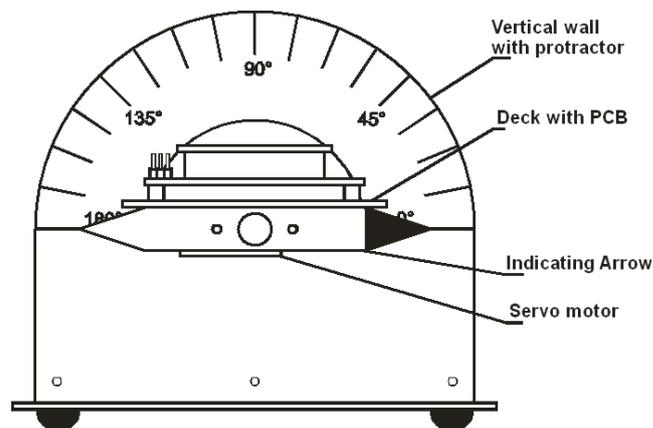
**Fig. 1 Mechanical construction of the stand**
