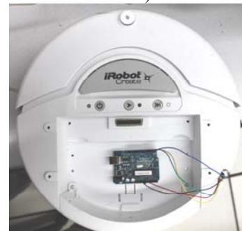
Figure 11: Hardware of ArEduBot system.
